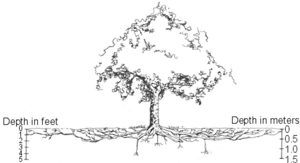
**The TPZ** is a radius 10 times the diameter of a tree measured at 4.5 feet above grade. The TPZ shall be determined the following way: the TPZ radius shall be 10 times the DBH (4.5') of the trunk. For example: a 15" DBH = a 12.5 foot radius from the perimeter of the tree, or a 25 foot **TPZ**. Any deviation in determining the **TPZ** shall be in accordance with ANSI standards subject to approval by the Town Arborist.
